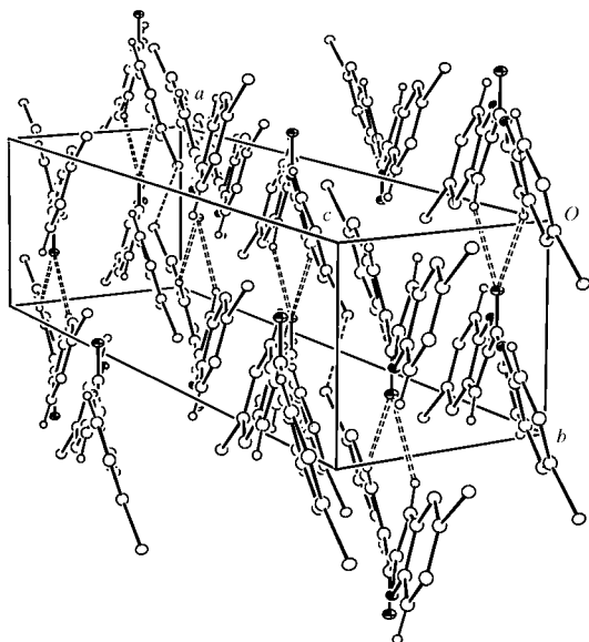
Figure 5 A packing diagram of (II). C—H...O interactions are represented as double dashed lines and Br...Br contacts are indicated by single dashed lines. O atoms are shown with octant shading.
